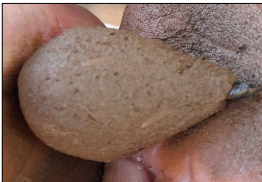
Fig.7 (b) Cover the mould again with red and yellow earth
