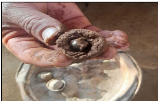
Fig.4 (a) Moulding on small ball with red earth, cow secrete sand
