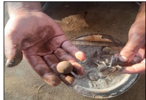
Fig.4 (b) Moulding on small ball with red earth, cow secrete sand
